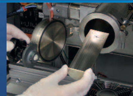
Operator loads Parylene precursor in Comelec coating plant.
