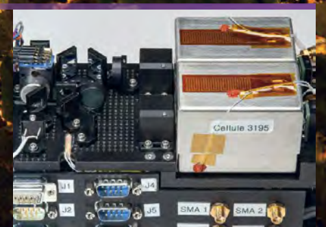
Highly-stable laser-pumped rubidium atomic clock developed at University of Neuchâtel
