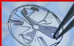
New single-piece oscillator in Zenith's «Defy Lab»
